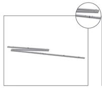
1. Start connecting the different sections of the frame by pushing the ends together.
