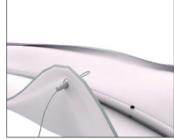
6.Thred cable support through eyelet.
