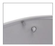
11.Pull the cable up through the eyelet to make if ready for the lift.
