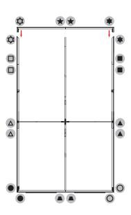
Push the silicone bead into each corner of the frame with your thumb.
