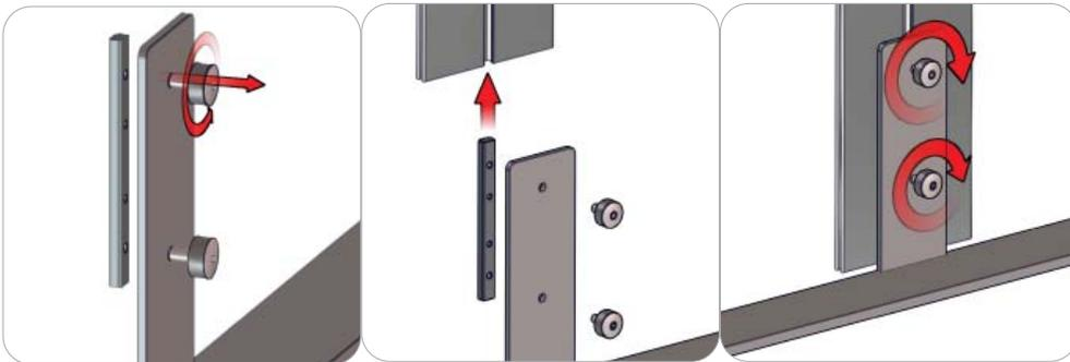
An SW-FOOT assembly consists of two thumb screws, an LN100, and SW-FOOT baseplate. Start by loosening the thumb screws (it is best not to completely remove the screws). Slide the extrusion onto the LN100 by utilizing its back cam channel. When the extrusion rests on baseplate or ground (depending on application), tighten the thumb screws to lock in place. Do not over tighten.
