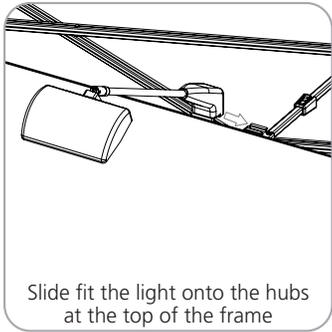
Slide fit the light onto the hubs at the top of the frame
