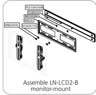
Assemble LN-LCD2-B monitor-mount
