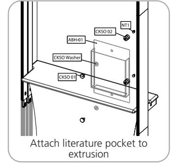
Attach literature pocket to extrusion
